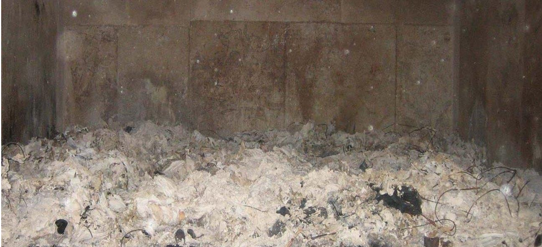
Ash from processing mixed MSW, I&C waste, the chamber was fully loaded with waste
