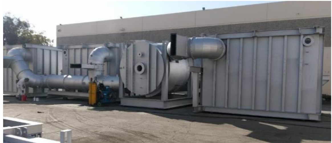
Combustion system major components during fit test at subcontractor's manufacturing site
